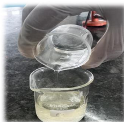
Fig 11:-Incorporation of water phase into oil phase
