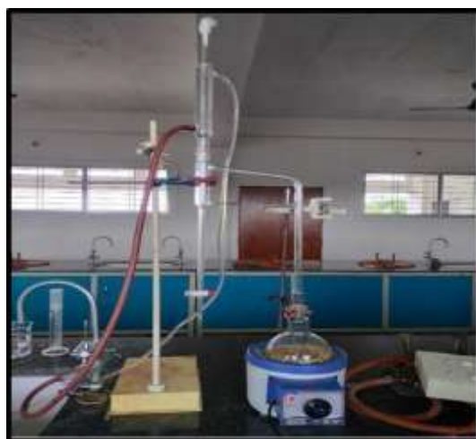
Fig 1. Extraction of Essential Oil by Clevenger Method
